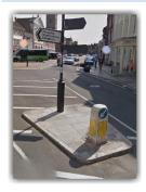
A pedestrian refuge island is a raised section of pavement between two lanes of traffic moving in opposite directions.
